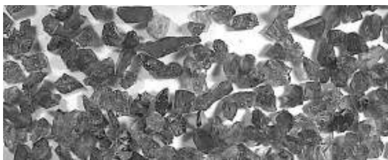
Figure 2. Product of electric pulse disintegration of garnet crystal, fraction -1 + 0.5
